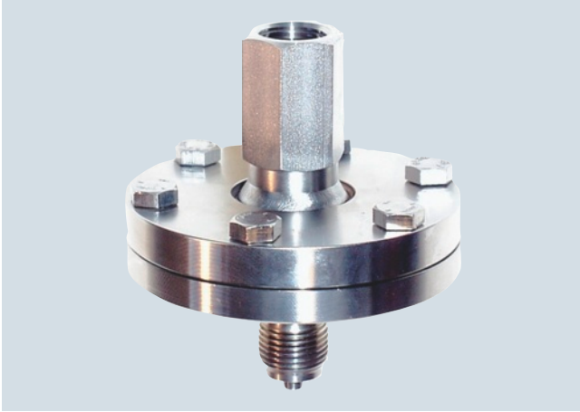
Diaphragm seal, screwed gland design with inside diaphragm for gauge, absolute and differential pressure for direct mounting
